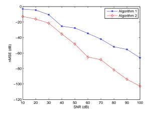
Fig. 5. Example 2: comparison of Algorithm 1 and Algorithm 2 on identifying the first two systems. The star-blue curve corresponds to the performance of Algorithm 1, while the diamond-red curve corresponds to the performance of Algorithm 2.
